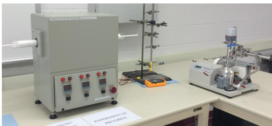
Fig. 2. Three-zone annealing furnace (shown on left-side) and vacuum pump (shown on right-side) for removing when sealing CdMnTe wafers in ampoules.
