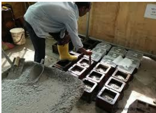
Figure3 it shows the preparation of hand mixing of concrete for compression strength of cubes. Figure 4 it shows the preparation of hand mixing of concrete for flexure strength of prisms.
