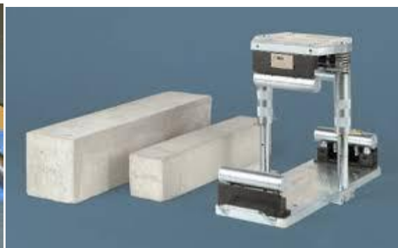
Figure 5 it shows the casting of the concrete cube. Figure 6 it shows the testing of flexure strength of prism.
