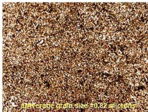
Figure 6: Microstructure of sand cast of 20 mm section size.
