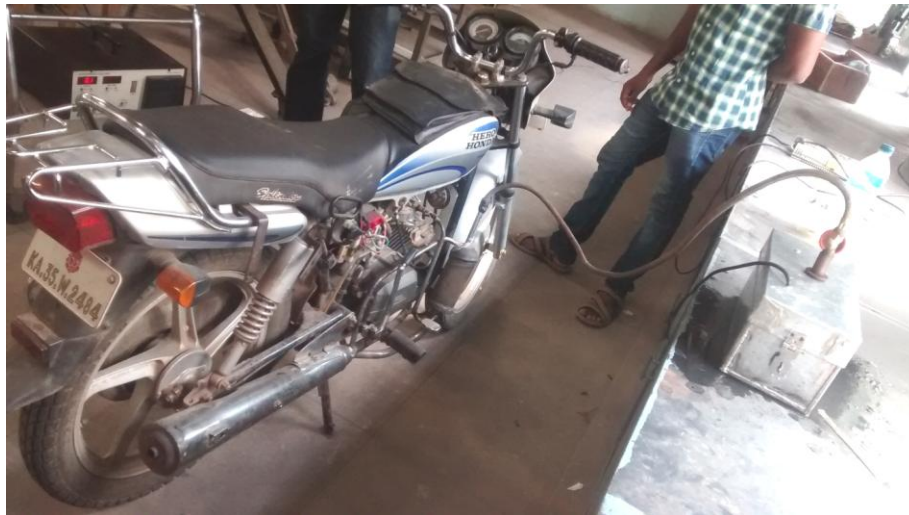
Fig-2. Basic setup for Emission testing
