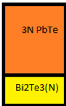
TE leg with two different materials
