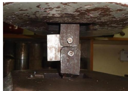
Figure 7: C(T) specimen loaded on UTM for fracture testing
