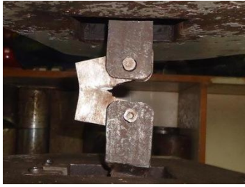
Figure 8(a): crack propagation commenced
