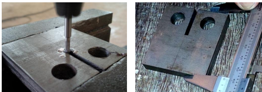
Figure 4: Compact Tension (C(T)) specimen made of SA-516 (before testing)
