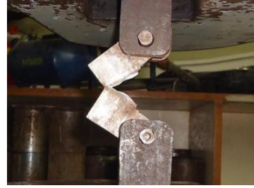
Figure 8(b): crack propagation advances
