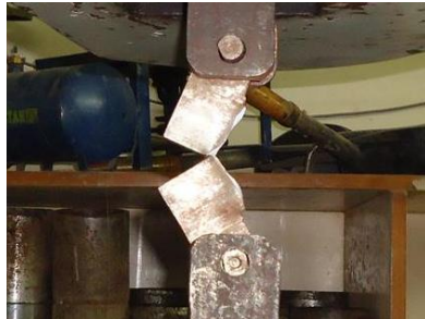
Figure 8(c): crack propagation reaches to full rupture
