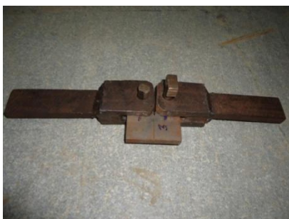
Figure 6: C(T) specimen with pin and fixtures
