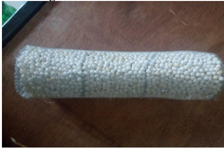
Figure 13 Wire mesh filled with Catalyst
