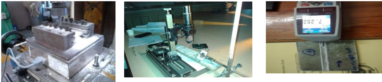
“Fig.”2.1. (a). Machining of GFRP laminate plate is properly fixed in machining center by special designed fixture located on mill tool dynamometer (b). Measurement of delamination damage using Travelling Microscope (c). Measurement of surface roughness by Mitutoyo Talysurf
