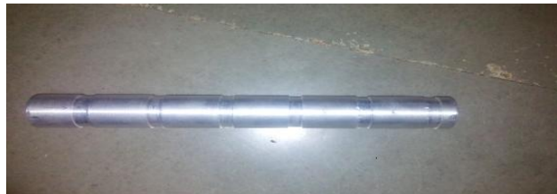
Fig 3 AL 6061 alloy Workpiece after Turning
