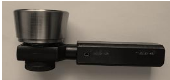
Fig 2 Single roller burnishing tool
