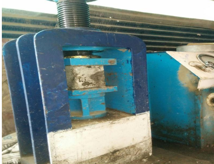
Fig.2 Compressive strength test setup
