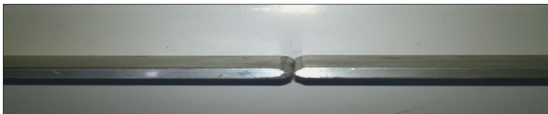
Fig.1 Specimen with double V groove joint
