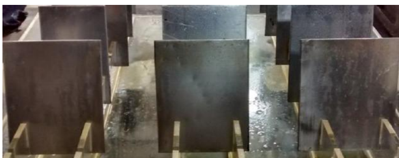
Fig 2: Salt spray test sample initial set-up
