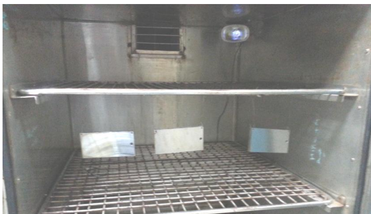
Fig1: Humidity chamber test set up
