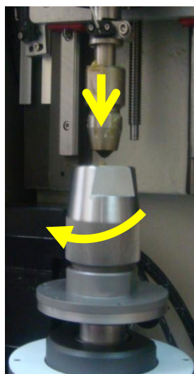
Fig 3: Four ball test arrangement
