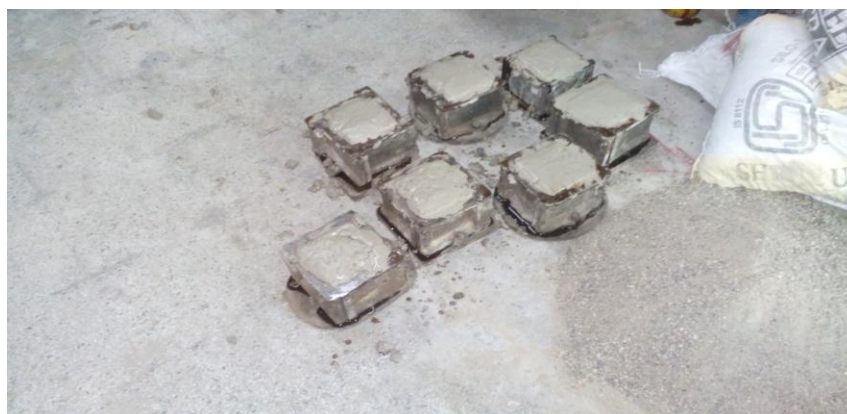
Fig: 1 sample casted into moulds.
