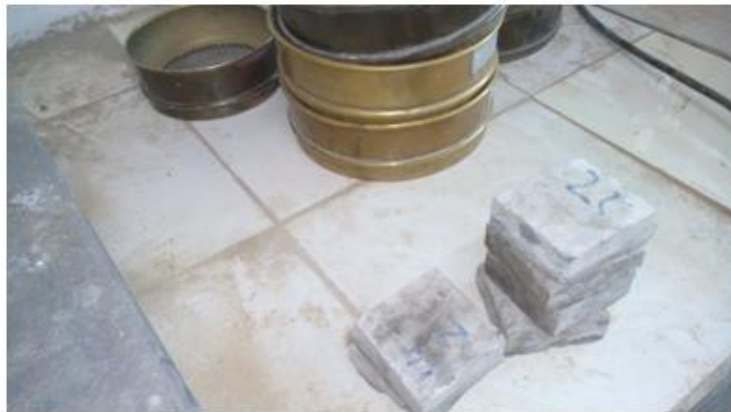
Fig 3 the samples are made of the required shape that can be fitted into the abrasion testing machine
