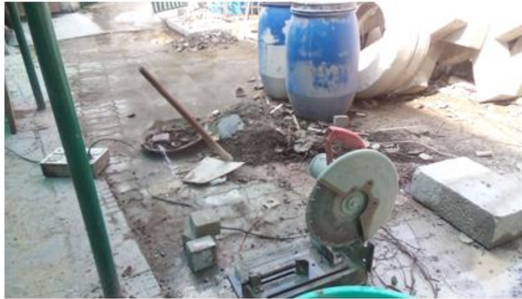
Fig 2 samples are cut into required size by the cutting machine
