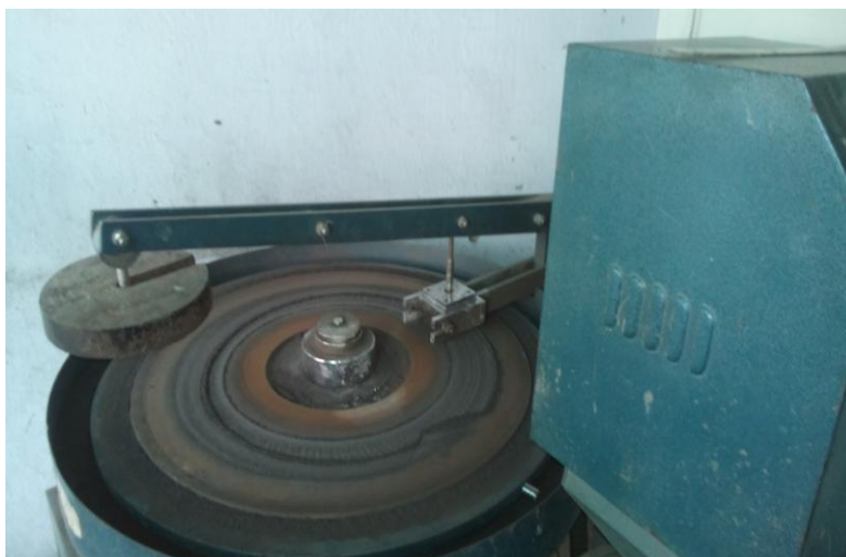
Fig 4 samples are fixed into the abrasion testing machine
