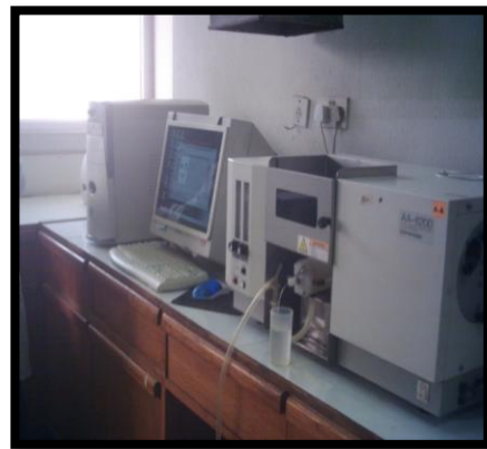
Fig. 4, the system used in evaluating of Pb concentrations in particulates (the atomic spectrum absorption system)
