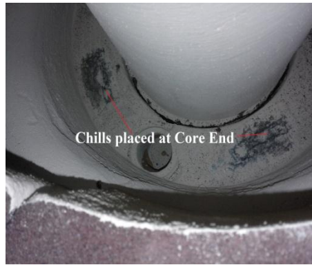
Fig.5. Chills Placing at Ends
