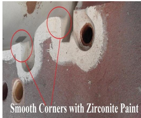
Fig.7. Smooth Corners with Zirconite Paint
