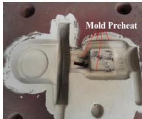
Fig.21.Mould Preheat at 45°C
