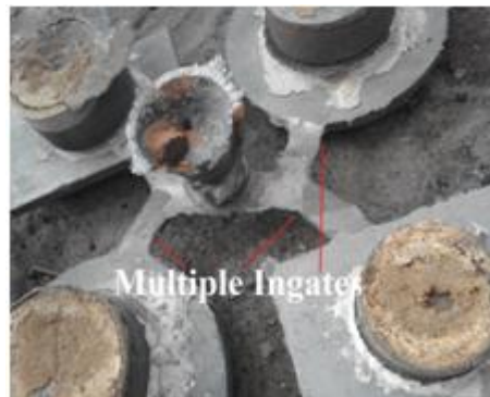
Fig.19. Multi Gates System
