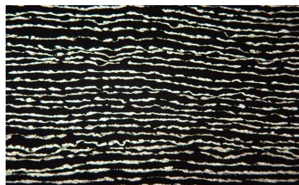
Transparent Concrete When Optical Fibres Are In Layered Distribution
