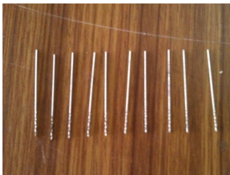
Fig 2 Micro drills with various point angle
