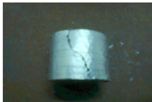
Fig 3.19 Compression Specimens After Test
