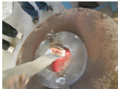
Fig 3.9 Adding reinforcent material Chopped Flyash Powder
