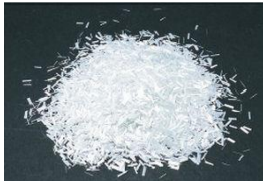
Fig 1.3 E-Glass Fiber Particles
