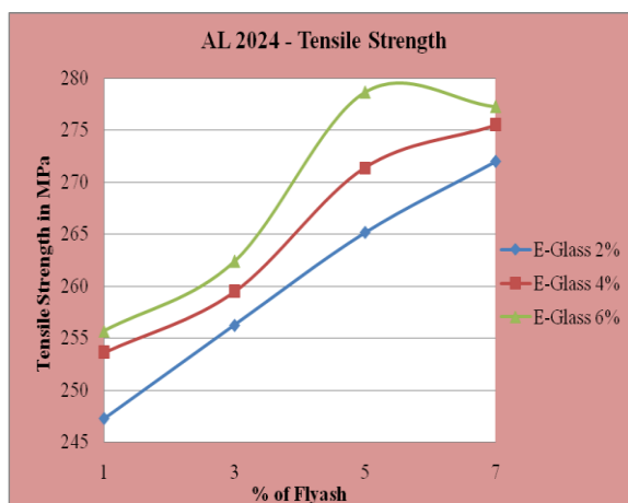
Graph 4.4: Comparative charts of Tensile test results for Al 2024 Hybrid Composites
