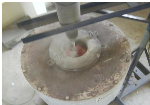
Fig 3.10 Stirring after Adding Reinforcements
