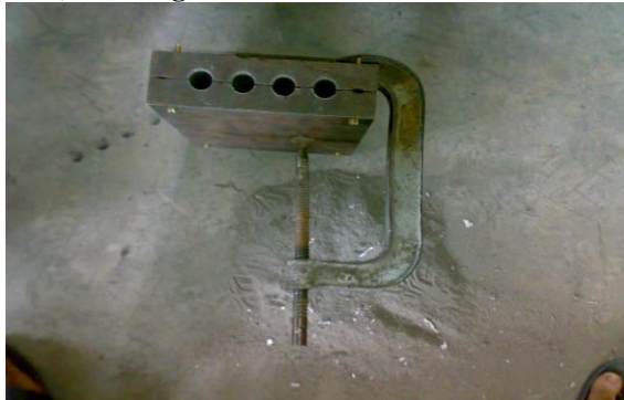
Fig 3.11 ASTM Mould Box
