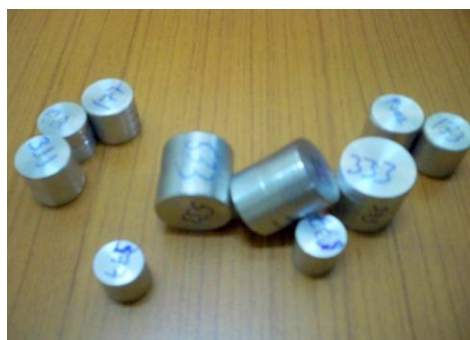
Fig 3.18 Compression Specimens Before Test
