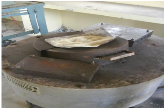
Fig 3.8 Adding reinforcent material Chopped E-Glass Fibre
