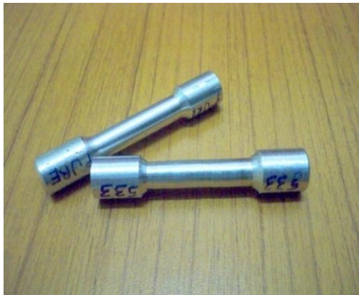
Fig 3.16 Tensile Specimens Before Test
