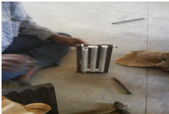
Fig 3.13 Removing Casted Component From Dies
