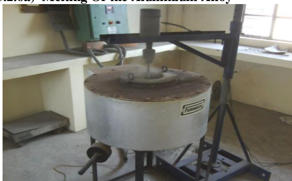
Fig 3.2 External View of Electrical Resistance Furnace
