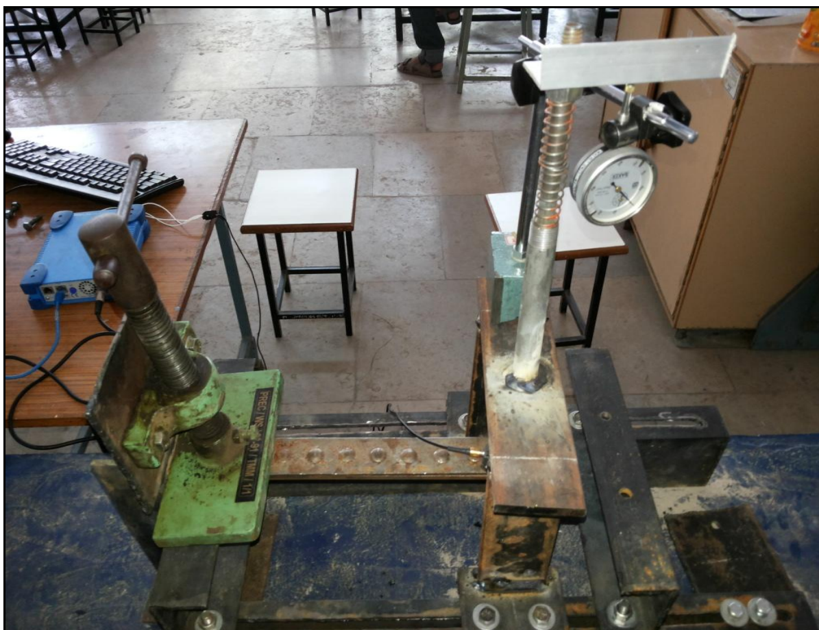
Fig.5: Side view of experimental set-up for cantilever beam
