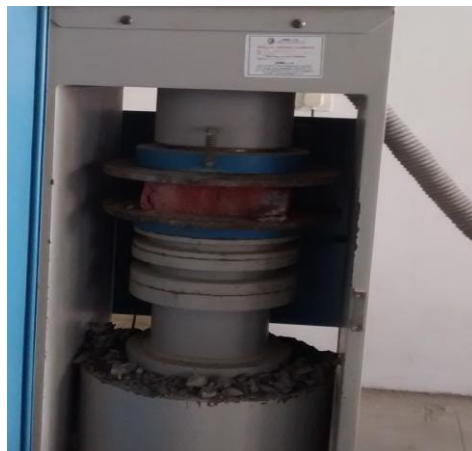
Figure 3 Compressive strength test
