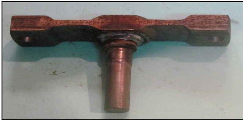
Fig. 11: Design of Yoke 18mm thickness for testing
