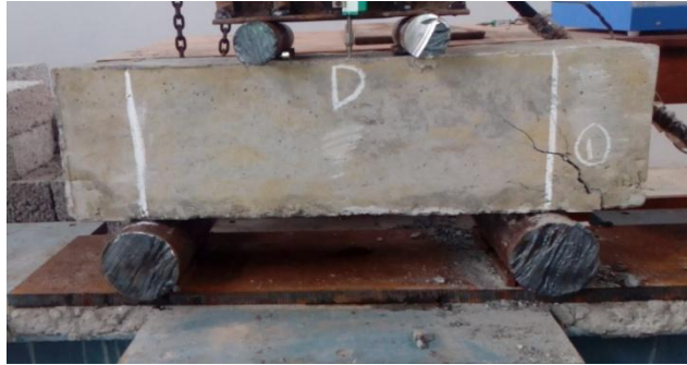
Fig.9. Crack Pattern of RSXB
