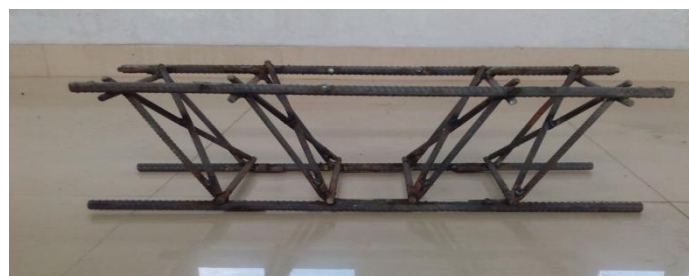
Fig.3. Reinforcement of Beam RSXB
