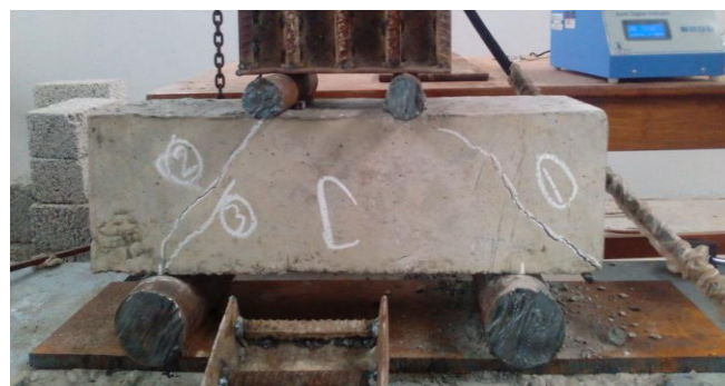
Fig.8. Crack Pattern of RSB
