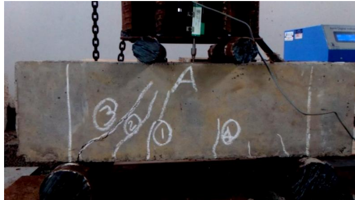
Fig.6. Crack Pattern of CB
