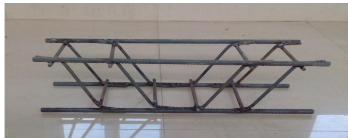
Fig.2. Reinforcement of Beam RSB
