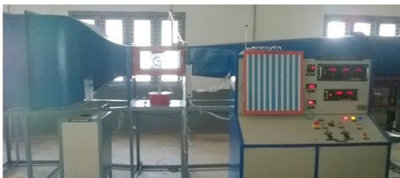
Fig 1. Low Speed Wind Tunnel
