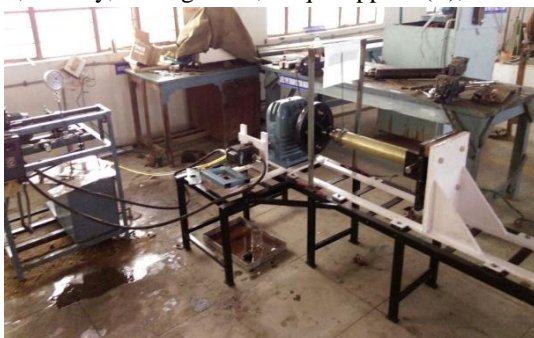
Fig.7 Hydraulic operated Torsion Testing Machine for Static Parameters
