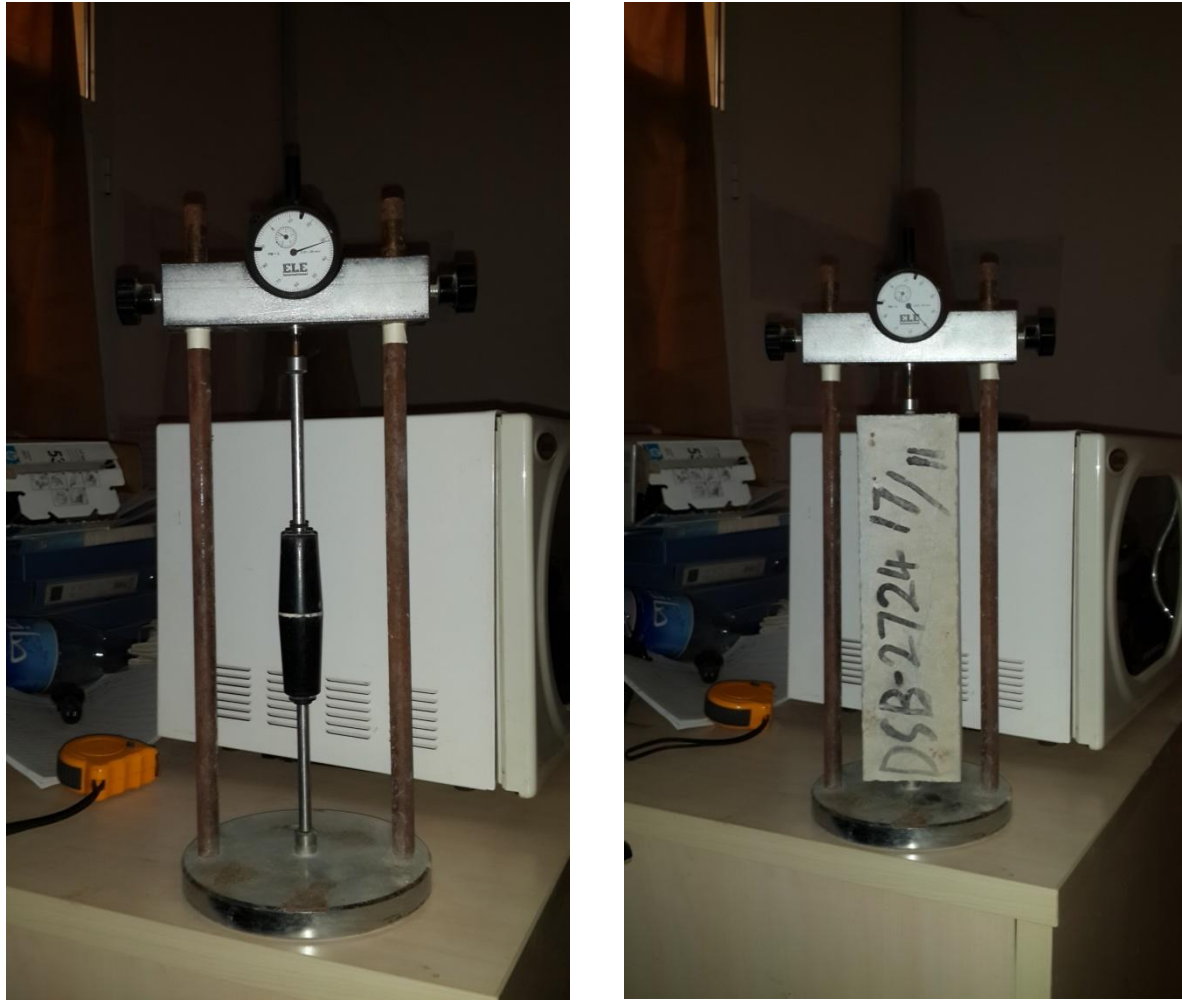
Figure(3): Shrinkage measuring apparatus along with calibration rod and specimen
