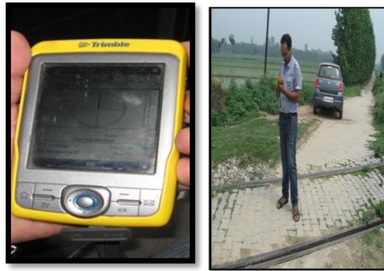
Fig. 3. GPS location data collection at unmanned railway crossings selected for the study.
