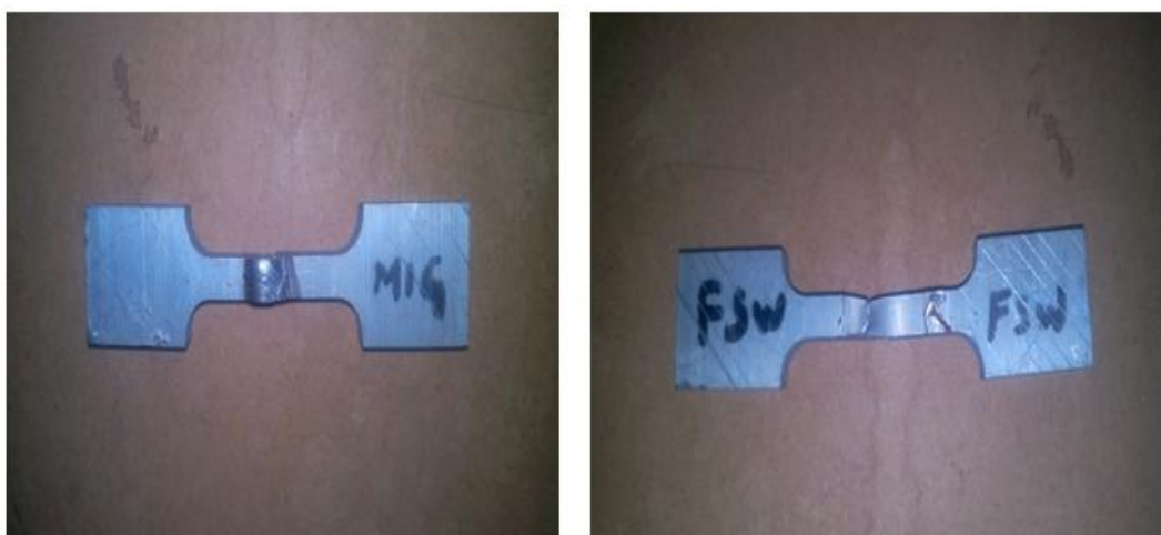
Fig.5. MIG and FSW welded plate Aluminium alloy tensile test specimen.
