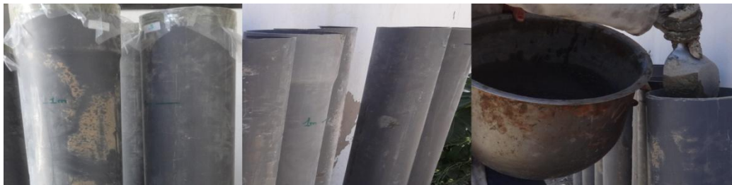
Photo 1. Closure PVC pipes with 5 cm mortar.
