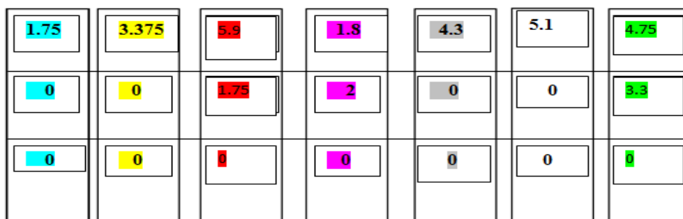
Figure. 5. Diagram showing the values of compressive strength in MPa obtained at the top, middle and basal piles SCC12 without colloid
