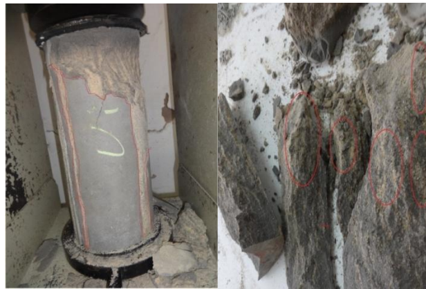
Photo 5: Structure of the specimen 5 after crushing
