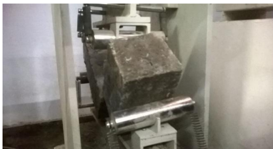
Fig. 3: Specimen after the application of load
