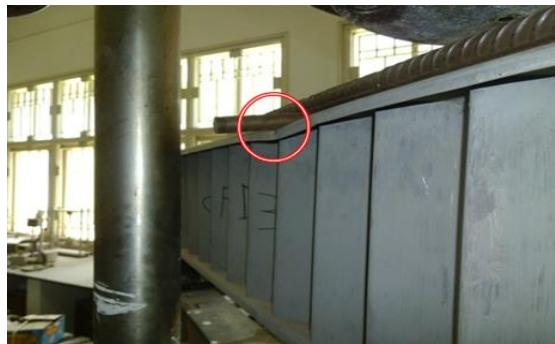
Fig. 5 Failure mode of test specimen- crushing on top flange.
