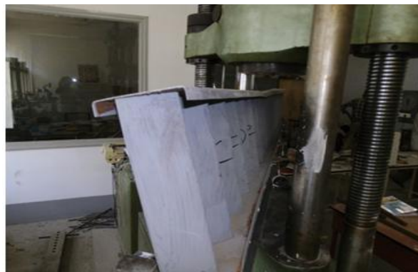
Fig. 6 Failure mode of test specimen- lateral torsional buckling.
