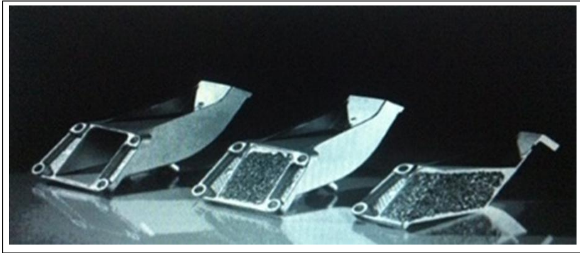
Fig.6 Prototype of BMW engine mounting bracket. From left: empty casting, composite part consisting of foam core and cast shell, and section through composite part.
