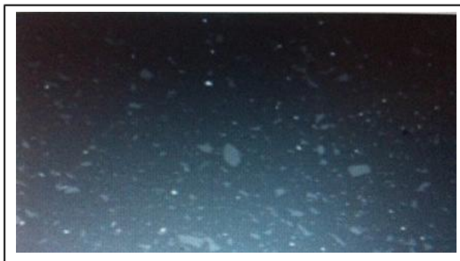
Fig.2. Foamable precursor sample of Al-alloys
