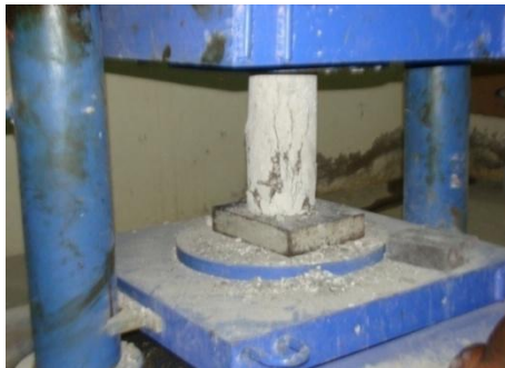
Plate 9. Test set up of Cylinder compressive strength
