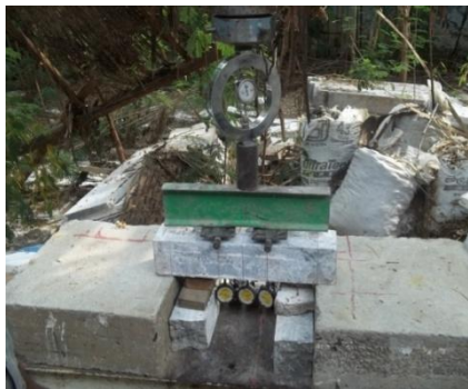
Plate 11. Test set up of beam for flexural strength
