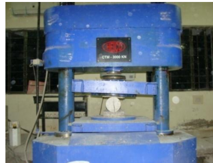
Plate 10. Test Set up of Split Tensile strength
