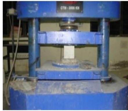
Plate 8. Test set up of cube compressive strength
