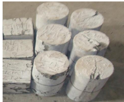
Plate 12. Crack patterns of specimens after testing.
