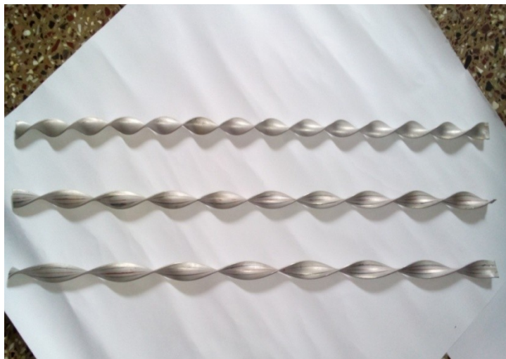
Fig. 2: Photograph of Twisted tape inserts
