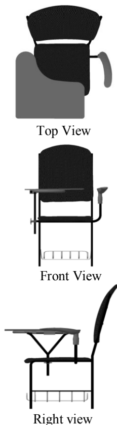
Fig 5.3: Orthogonal view of Proposed Tabloid chair.
