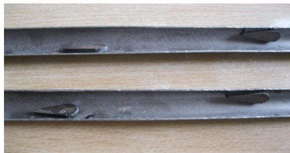
Fig.5: Photograph of Test tube section with cross dimple array
