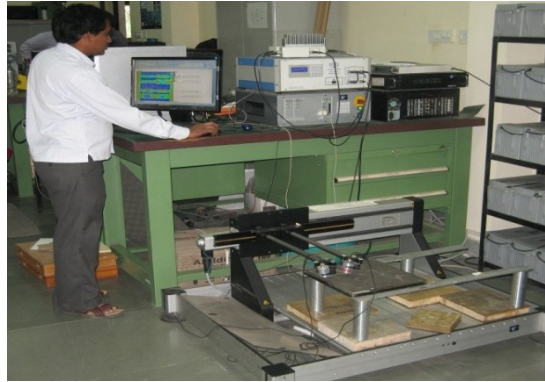
Figure1a: Complete experimental arrangement consisting of Ritec Pulsar Receiver system, XY scanner for c-scan imaging system, Ultrason air coupled Transducers-glass laminate.
