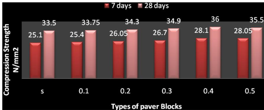
**Fig.No.4. Compressive strength at 7 & 28 days for Paver blocks without and with fibers**
