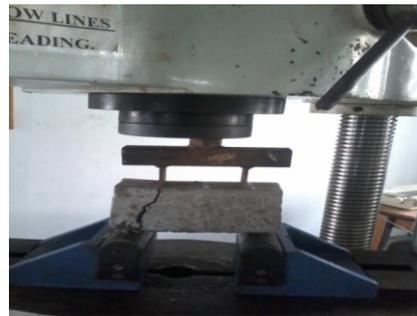
**Fig .No.3. Flexural strength test**
