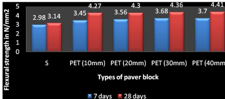
**Fig .No.8. Flexural strength of paver block at 0.4% fiber by changing top layer thickness**
