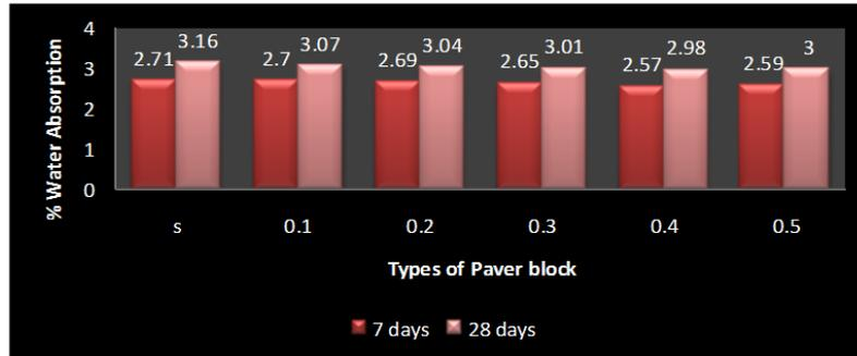
Fig .No.5. Water absorption at 7 & 28 days for Paver blocks without and with fibers
