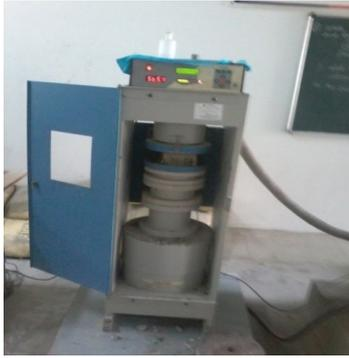
**Fig . No.1. Compressive strength test**
