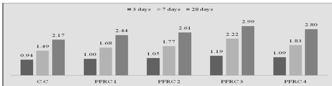
Fig.no.6:- Type of mix vs. Split tensile strength (N/mm<sup>2</sup>) at 3, 7 & 28 Days
