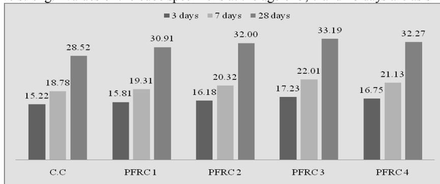
Fig. No.5:- Type of mix vs. Compressive strength (N/mm<sup>2</sup>) at 3, 7 & 28 Days
