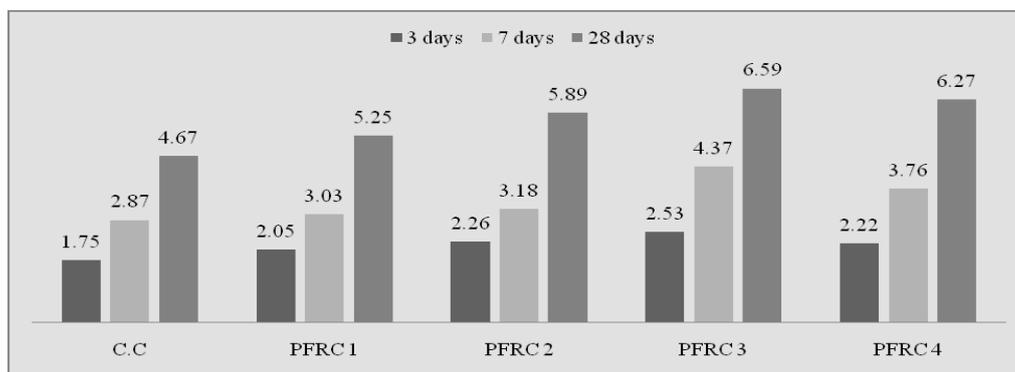
Fig.no.7:- Type of mix vs. Flexural strength (N/mm<sup>2</sup>) at 3, 7 & 28 Days
