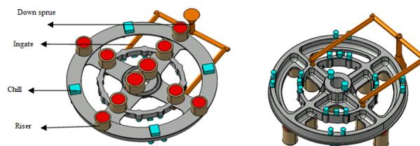
Fig: 2 Top & bottom view of f Flywheel (modified model)
