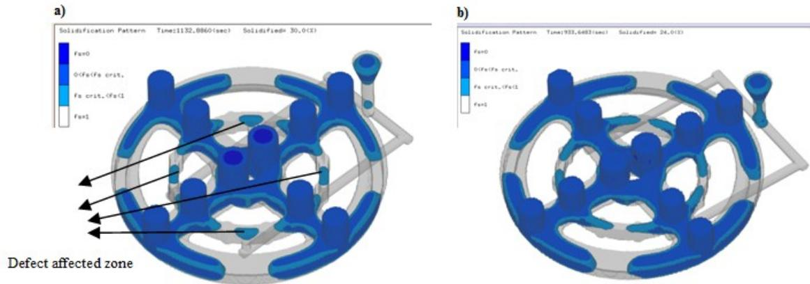
**Fig: 4** Solidification of the casting component.
