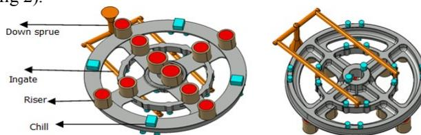
Fig: 1 Top & bottom view of f Flywheel
