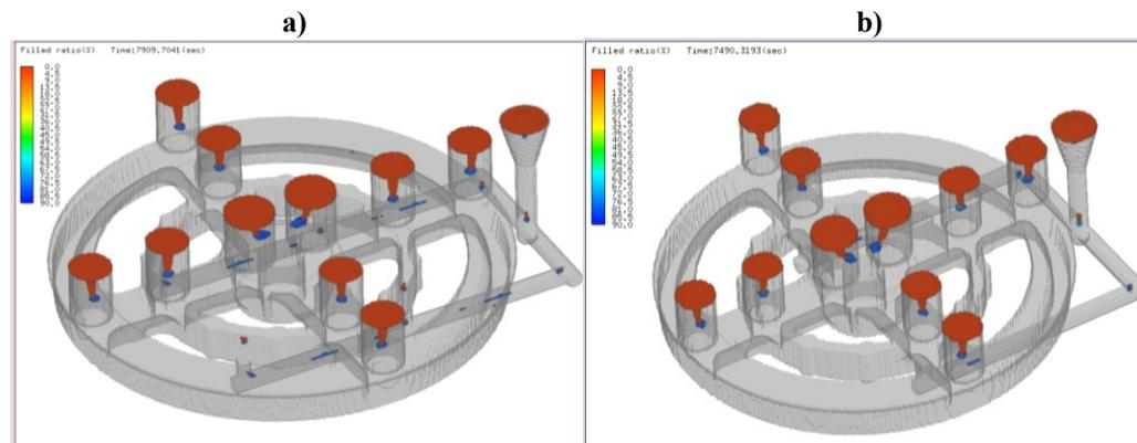
**Fig: 5** Shrinkage porosity in the casting component.
