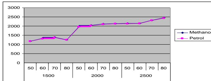
Fig.4.18 The effect of engine coolant temperature on NOx emission with varying engine speed and at an engine load of 12 kg
