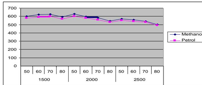
**Fig.4.3** The effect of engine coolant temperature on specific fuel consumption with varying engine speed and at 12 kg engine load.
