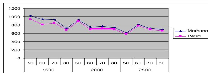
**Fig.4.1** The effect of engine coolant temperature on specific fuel consumption with varying engine speed and at 6 kg engine load.
