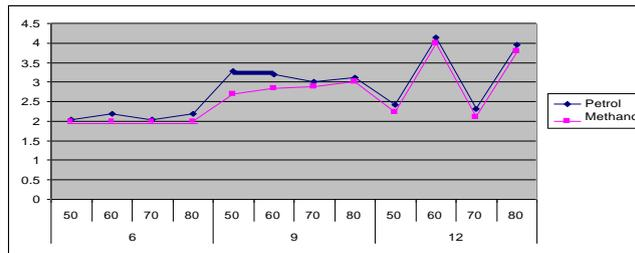
Fig.4.10 The effect of engine load on brake power with varying engine coolant temperature and at an engine speed of 1500 rpm
