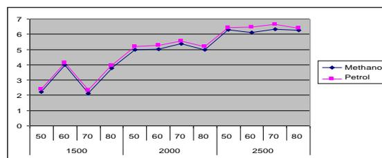
**Fig.4.6** The effect of engine coolant temperature on brake power with varying engine speed and at 12 kg engine load.
