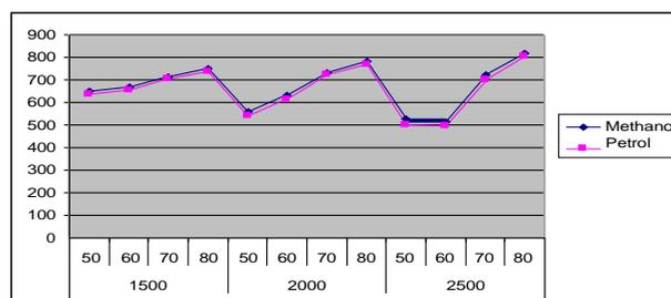
Fig.4.16 The effect of engine coolant temperature on NO<sub>x</sub> emission with varying engine speed and at an engine load of 6 kg
