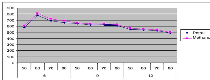
Fig.4.9 The effect of engine load on specific fuel consumption with varying engine coolant temperature and at an engine speed of 2500 rpm
