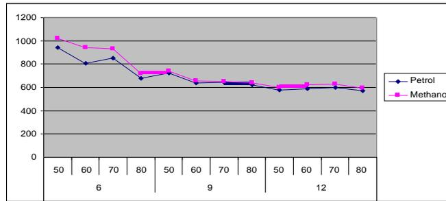
Fig.4.7 The effect of engine load on specific fuel consumption with varying engine coolant temperature and at an engine speed of 1500 rpm
