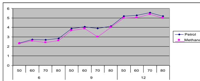
Fig.4.11 The effect of engine load on brake power with varying engine coolant temperature and at an engine speed of 2000 rpm
