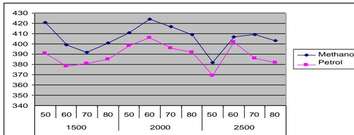
Fig.4.14 The effect of engine coolant temperature on HC emission with varying engine speed and at an engine load of 9 kg
