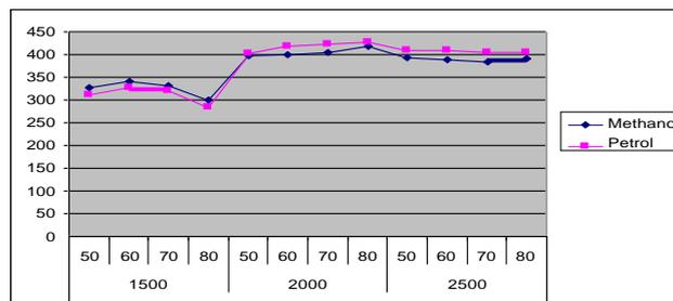
Fig.4.15 The effect of engine coolant temperature on HC emission with varying engine speed and at an engine load of 12 kg
