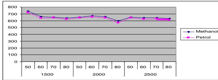
**Fig.4.2** The effect of engine coolant temperature on specific fuel consumption with varying engine speed and at 9 kg engine load.
