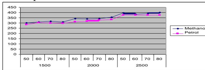
Fig.4.13 The effect of engine coolant temperature on HC emission with varying engine speed and at an engine load of 6 kg
