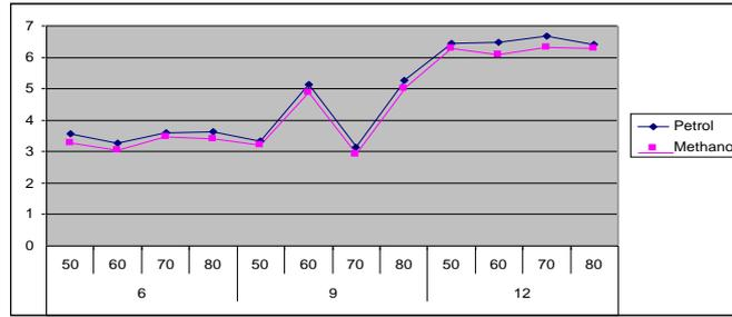
Fig.4.12 The effect of engine load on brake power with varying engine coolant temperature and at an engine speed of 2500 rpm
