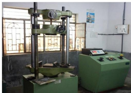
**Figure 1:** Universal Testing Machine
