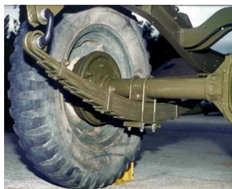
Figure 1(a): Shows a truck equipped with leaf spring.
