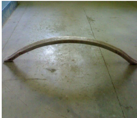
Figure 5(b) Specimen of composite leaf spring. (K. K. Jadhao et al 2011)
