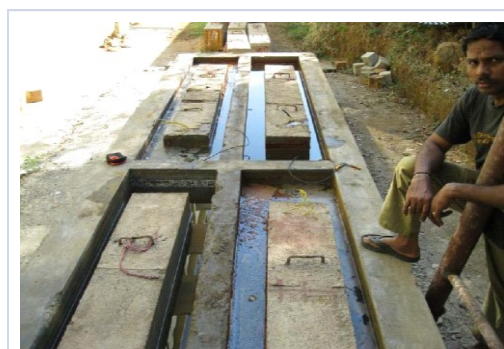
Fig.4.7.1 Photo of beam specimens under accelerated corrosion
