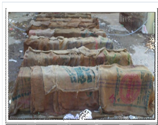
Fig.4.6.2 Curing of Beam Specimen
