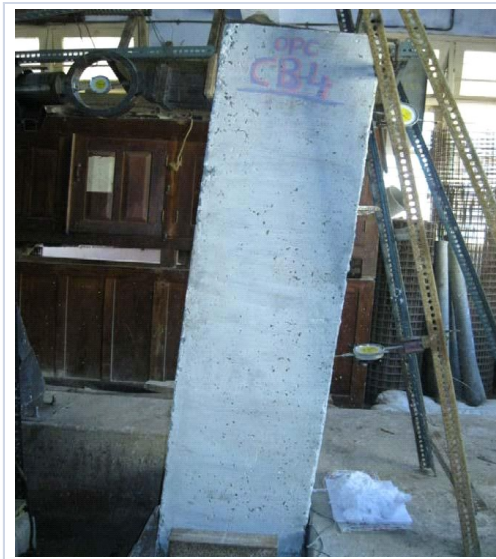
Fig.6.2 Deflection of beam after Flexure failure
