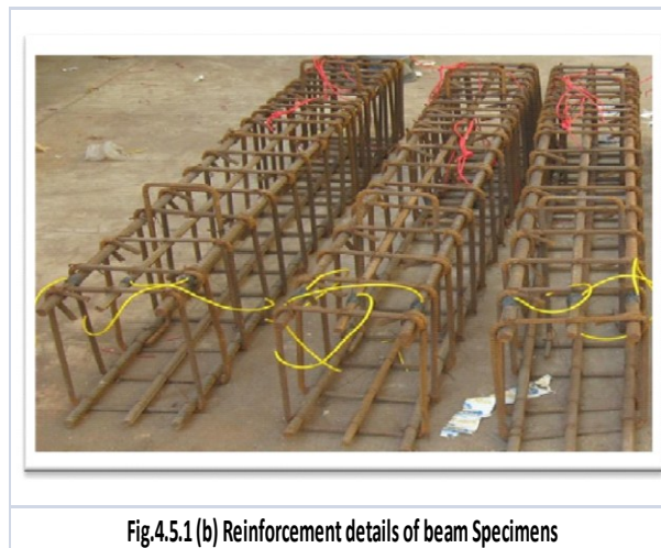
Fig.4.5.1 (a) Reinforcement details of beam specimens
