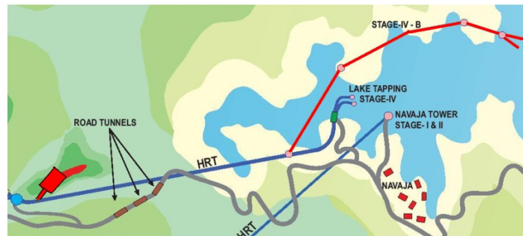
Fig.2.1.1 Schematic drawing of lake tapping at stage-4 th and stage-4 th B in Koyna Dam
