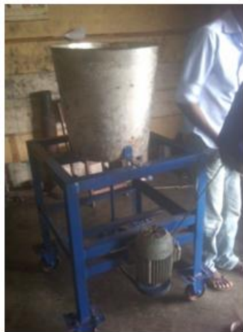
Figure 8: Finished de-feathering machine
