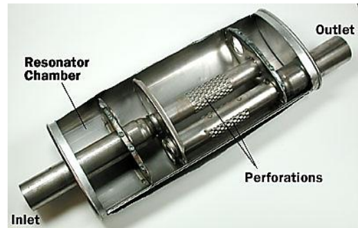
Figure 2 Reactive Muffler[2]
