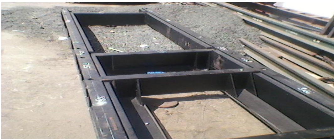
Figure 2.3 Rail engine alternator set base frame
