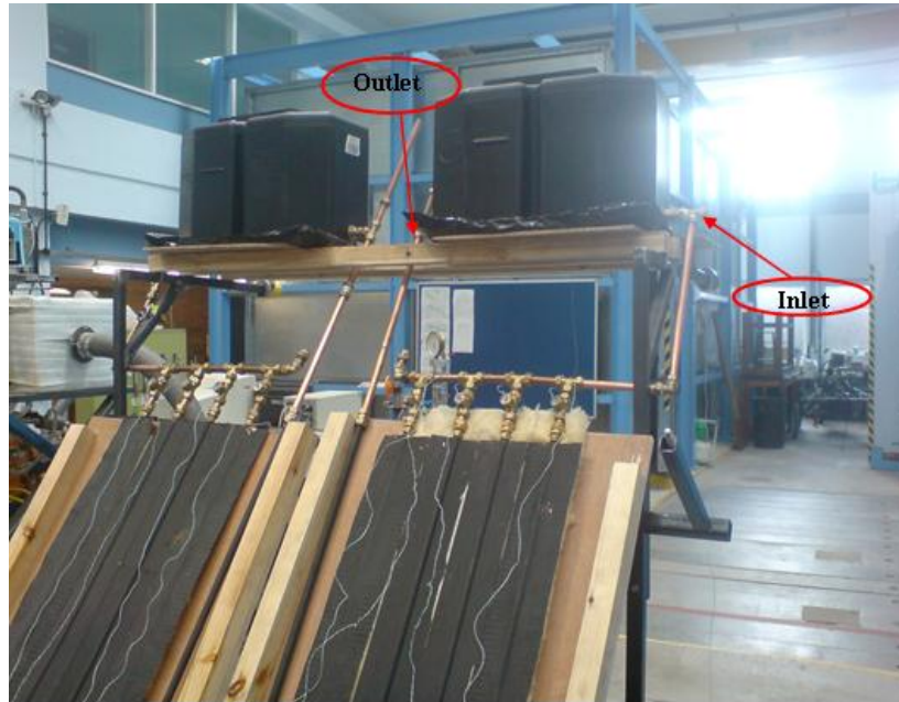
Fig. 2. Water tanks connected to the collectors.
