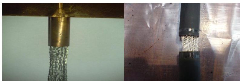
Fig. 1. Aluminium mesh inserted in copper pipe.
