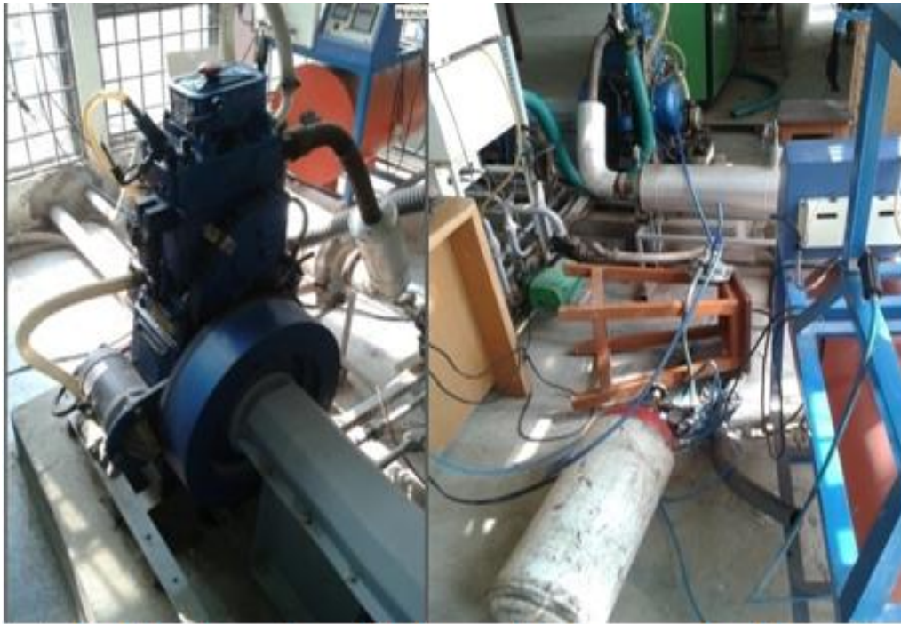
Fig.1 Single cylinder, four stroke, multi-fuel, research engine connected to eddy type dynamometer
