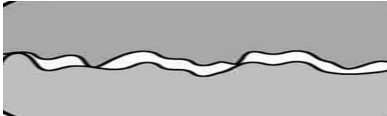
Figure 4: Microscopic view of two surfaces in contact
